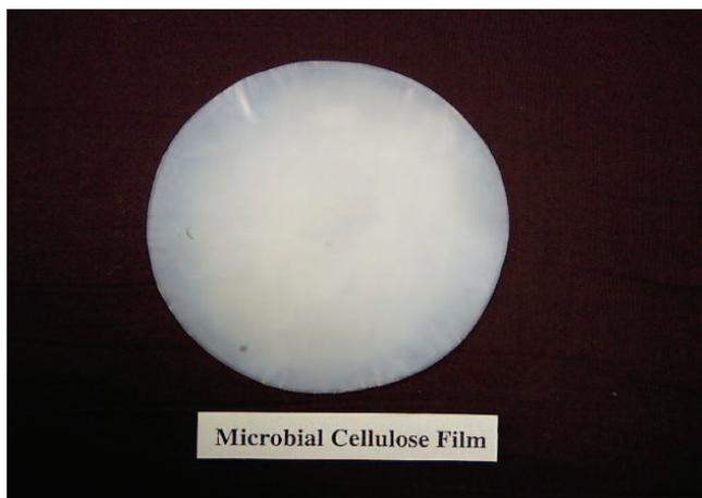
Figure 3. Photograph of membrane prepared from chemically treatment of MC pellicle.
