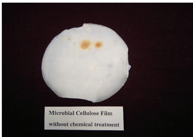
Figure 4. Photograph of membrane prepared without chemically treatment of MC pellicle
