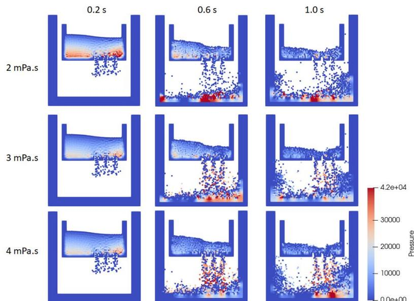
**Figure 2.** Pressure profile on dynamic viscosity variation
