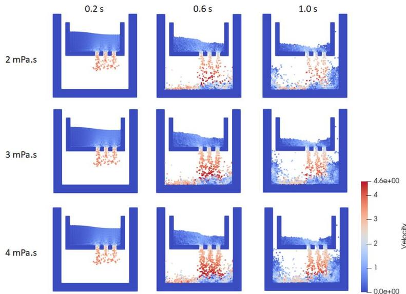
**Figure 3.** Velocity profile on dynamic viscosity variation
