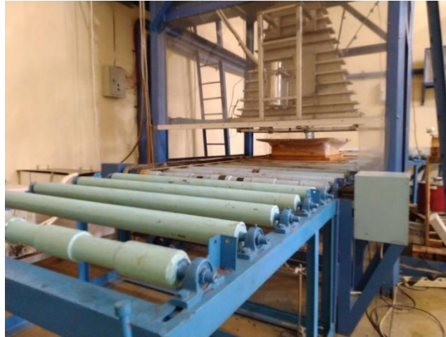
Figure 1. Conveyor system for irradiation in Arjuna 1.0
