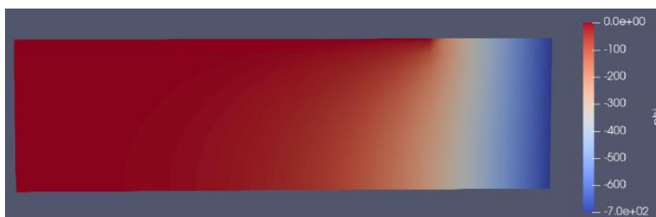
Figure 5. Electric potential distribution inside the ion chamber
