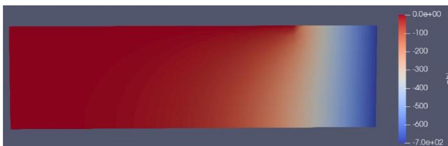
**Figure 5.** Electric potential distribution inside the ion chamber
