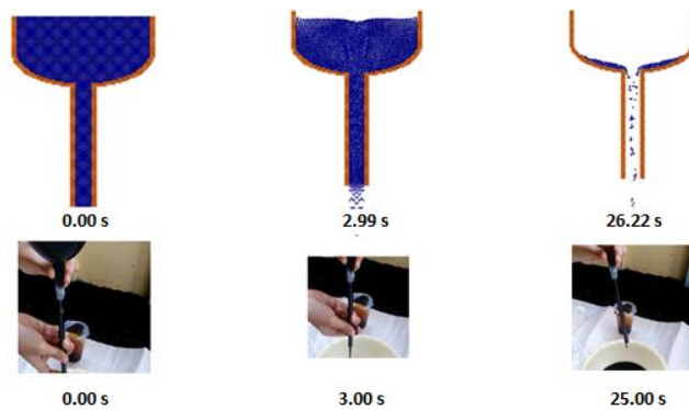
Figure. 6. Comparison of time of oil flow between simulation and experiment.
