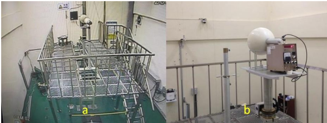
Figure 12. (a) KRISS neutron calibration room, and (b) measurement of ^{252}\text{Cf} neutron spectra using BSS
