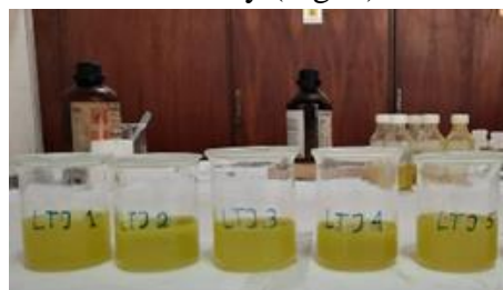
Figure 1. Precipitation of REE oxide using oxalic acid
