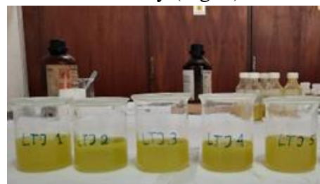
Figure 1. Precipitation of REE oxide using oxalic acid
