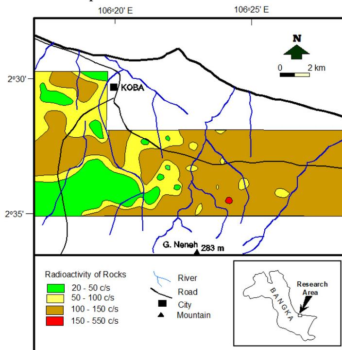
Figure 4. Radioactivity of the Rocks in Koba Area, Central Bangka [11].
