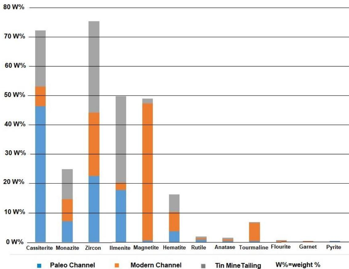
Figure 3. The average mineral content of pan concentrates in paleochannels, modern channels, and tin mine tailing deposits (data taken from [11]–[13]).
