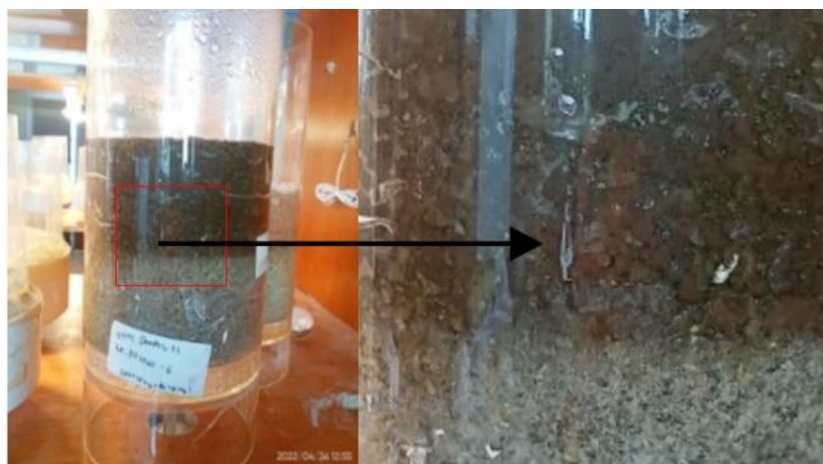
Figure 8. Gaps formed due to fly ash grains clumping together.
