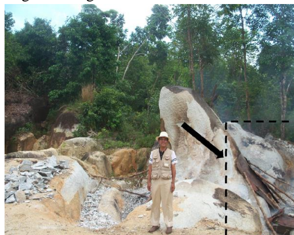
Figure 4. A traditional granite mining sites on Belitung Island. Miners need to heat the granite so it is easier to be cut
