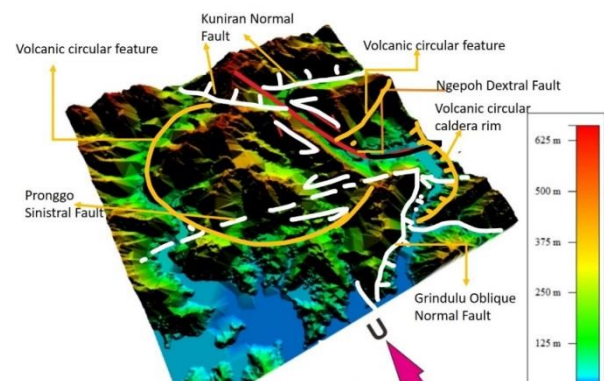
Figure 2. The Digital Elevation Model (DEM) of the research area, shows the geomorphology of circular hills of volcanic origin that have been strongly slashed.
