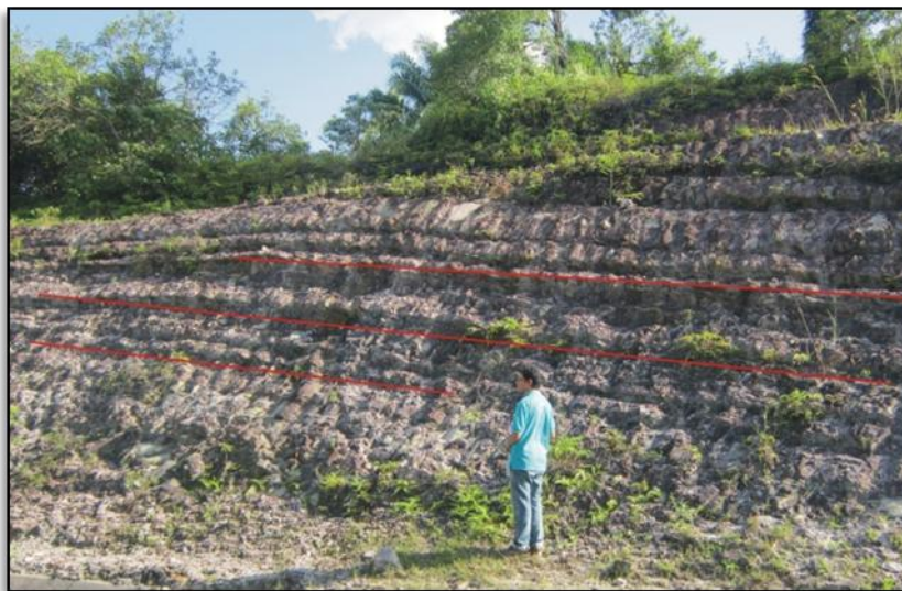
Figure 7. Photograph shows one parallel bedding planes in location 4 which is striking SE ( 107^\circ ) with gently dipping around 26^\circ towards southwest
