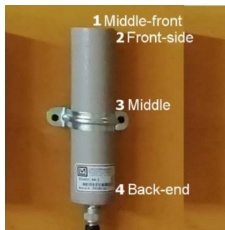
Figure 3. The GAM Detector and Source Position for Radiation Measurement
