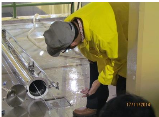
Gambar 1. Tabung uji cicip/sipping tube
