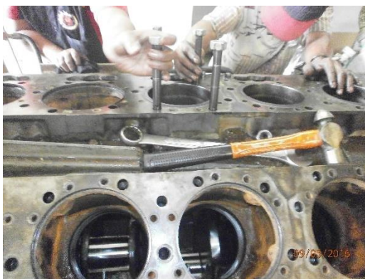
Gambar 4c: Lubang linner korosi
