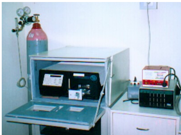
Gambar 13. Alat cacah sistim alfa/beta total, model MPC-9400
