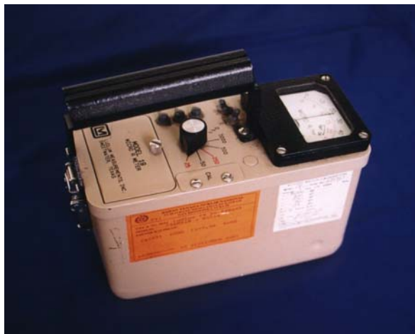
Gambar 8. Survey meter gamma micro R meter model 19, Ludlum-USA
