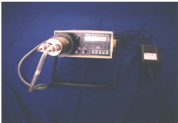
Gambar 6. Monitor radon – thoron model AB-5 Pylon Inc. Canada
