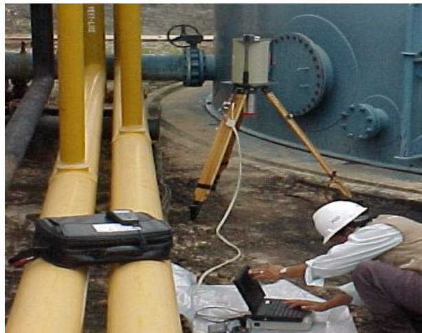
Gambar 11. Spektrometer gamma In situ detektor HPGe model GC2020, Canberra – USA
