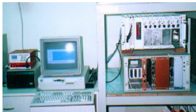
Gambar 12. Spektrometer alfa detektor silicon surface barrier , Tennelec - USA
