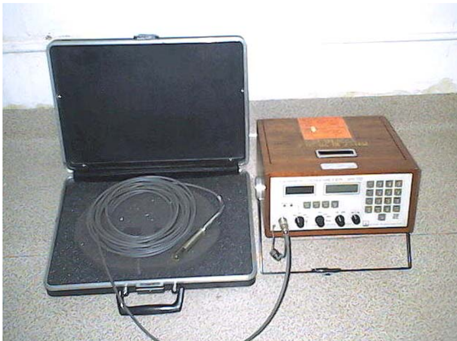
Gambar 2. Alat Ukur Standar Dosimeter Farmer
