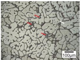
Figure 3. Optical microstructure of as received Al-SiC composite.
