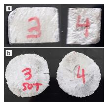
Figure 1. The sample of Al-Si composite. (a) Before forging; (b) After forging.
