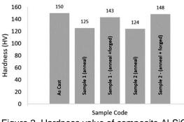
Figure 2. Hardness value of composite Al-SiC.
