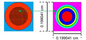
Figure 2. Visualization of kernel plated TRISO in the form of SC lattice on pebble fuel using Vis Ed program
