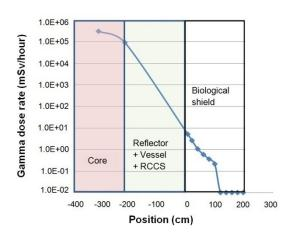
Figure 7. Relation of gamma dose rate in the core and the thickness of shielding the HTGR-10 MWth
