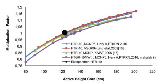
Figure 5. Calculation of core criticality on HTGR-10MWt and HTR-10
