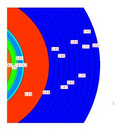
Figure 4. Visualization biological shield modeling by using MCNP6
