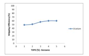
Figure 6. Correlation of % TOPO-kerosene and stripping efficiency
