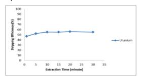
Figure 15. Correlation of extraction time (minute) and stripping efficiency
