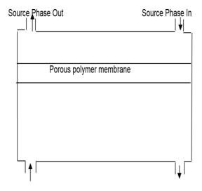
Figure 2. Configuration supported liquid membrane
