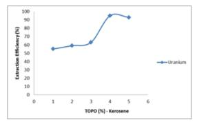
Figure 5 : Correlation of % TOPO–Kerosene and extraction efficiency
