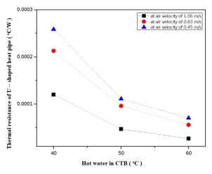
Fig. 5. The resistances of thermal of UHP[16]
