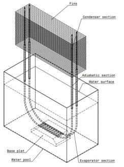
Fig. 2. Large geometry of UHP as PCS in CT
