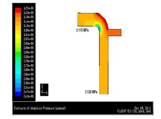
Fig. 5. Pressure contour at inlet the pressure of 3.120 MPa
