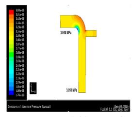
Fig. 3. Pressure contour at the inlet pressure of 3.050 MPa
