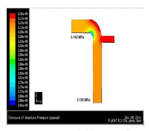
Fig. 6. Pressure contour at the inlet pressure of 3.150 MPa
