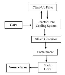
Fig. 1. Mechanism Transport of source term at normal operation of PWR-100MWe
