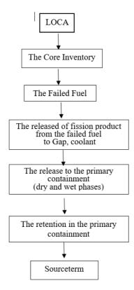
Fig. 2. Transport mechanism of source term at LOCA of PWR-100MWe
