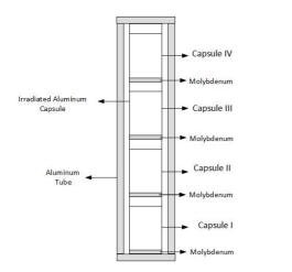
Fig. 14. Stacking irradiated aluminum capsule in aluminum tube
