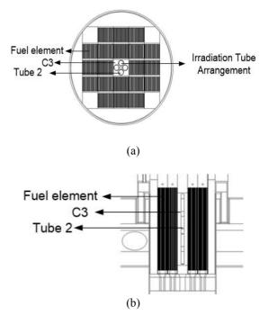
Fig. 11. Reactor core model configuration 2; (a) Cross section at xy-axis, (b) Cross section at xz-axis
