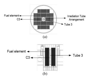
**Fig. 12**. Reactor core model configuration 3 (Cross section at xy axis (a), Cross section at xz axis (b) )
