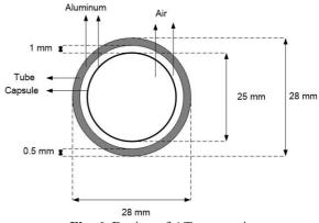
Fig. 6. Design of AT at xy axis
