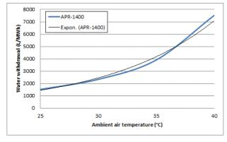
Fig. 10. Relationship between water withdrawal of NPP and ambient air temperature.
