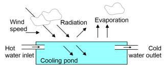
Fig. 7. Cooling pond mechanisms.
