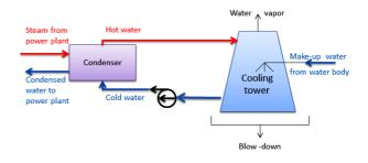
Fig. 3. Diagram of cooling tower system.
