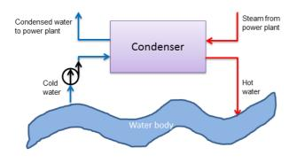
Fig. 2. Diagram of once through cooling system.
