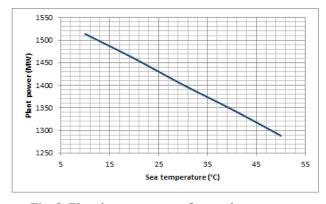
Fig. 8. Electric power output for varying sea water temperatures (modified from [11]).
