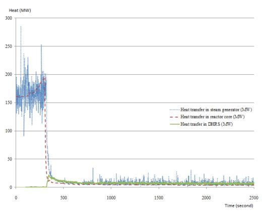
Figure 5. Heat transfer in the core, steam generator and DHRS.
