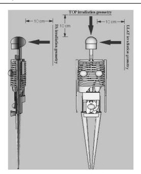
Figure 1.Outline and irradiation geometries of the ORNL MIRD phantom.
