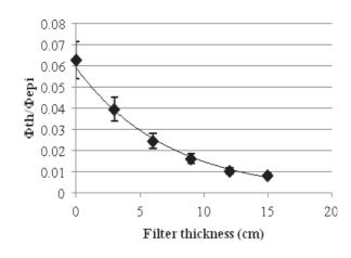
Figure 4. Thermal neutron component for various thickness of filter (60Ni).
