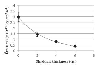
Figure 5. Gamma-ray component for various thickness of shielding (Bi).
