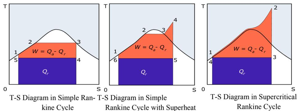
Figure 1. T-S Diagram of Rankine Cycle [18]
