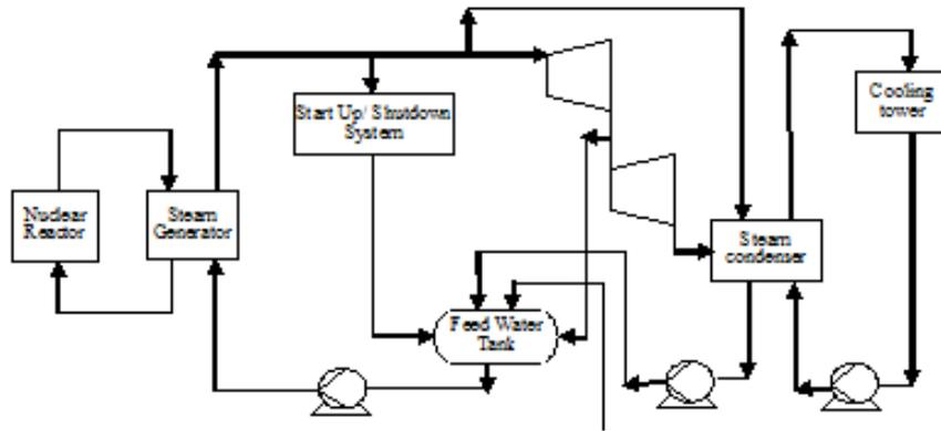
Figure 2. Schematic of RDE Cooling System [20]
