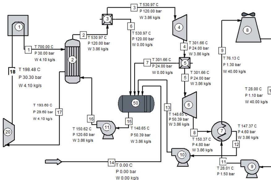
Figure 3. Model of RDE Cooling System Using ChemCAD
