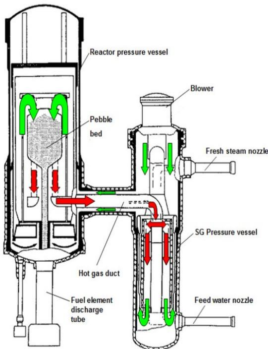
Fig. 1. Schematic Flow Diagram of Nuclear Steam Supply System<sup>[13]</sup>
