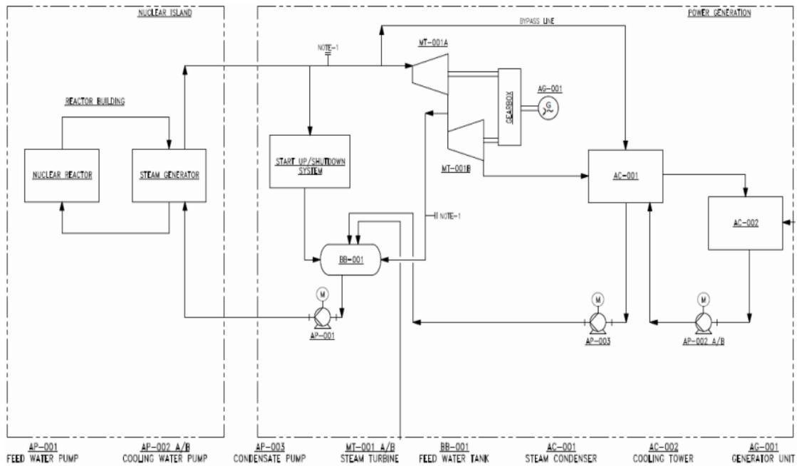
Fig. 2. Schematic of RDE cooling system [18]
