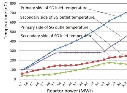
Fig. 5. Steam generator inlet and outlet temperatures on the primary and secondary side as function of reactor power
