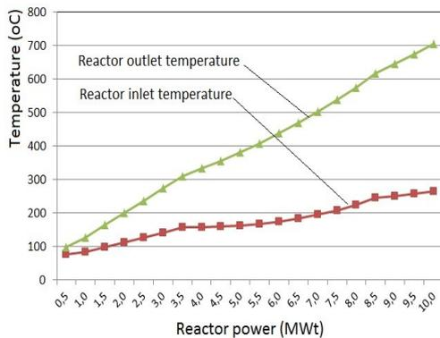
Fig. 4. Temperature of inlet and outlet reactor as function of reactor power
