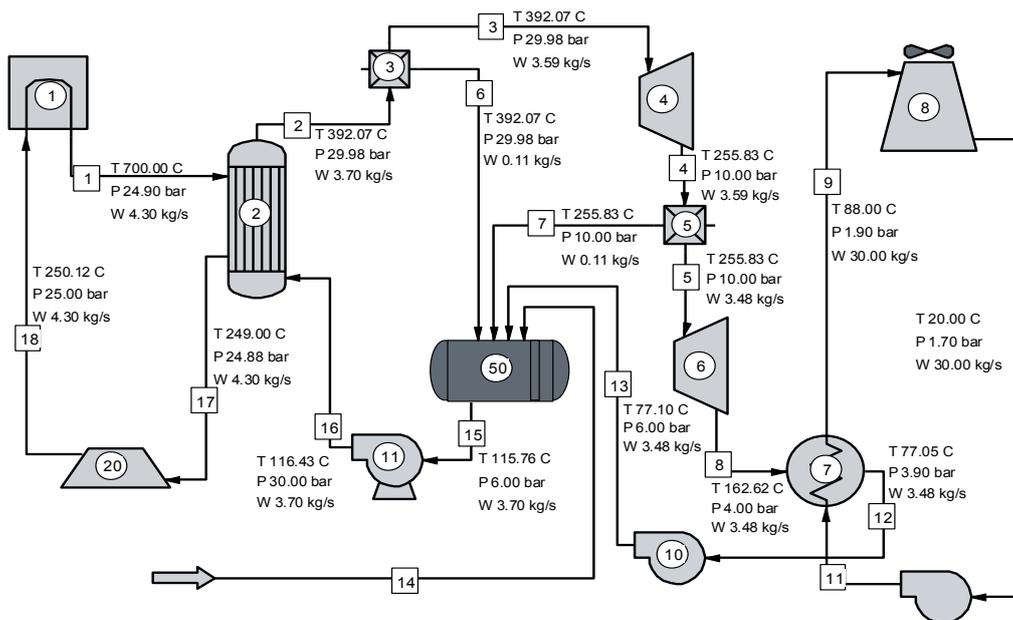
Fig. 3. Model of RDE cooling system using CHEMCAD
