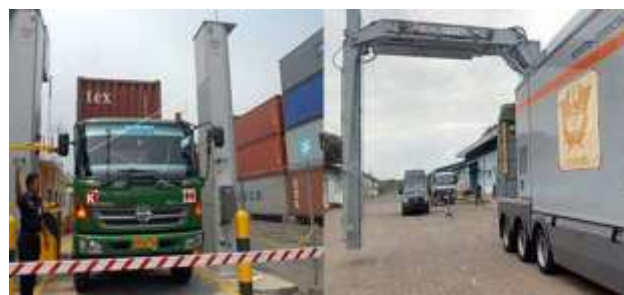
Figure 2. VACIS Gamma Ray Scanner installed in Tanjung Perak, Surabaya Indonesia [14] .
