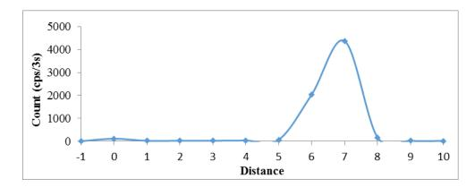
Figure 1. Chromatogram of lodine-131 using whatman No. 1 paper as stationary phase and methanolwater (80:20) as mobile phase.
