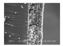
Figure 4. Cross-section of TiO<sub>2</sub> film on glass substrate
