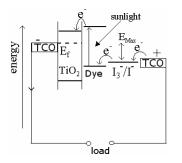
Figure 1. Principle of dye sensitized solar cell
