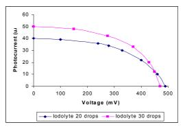
*Figure 7.* I-V characteristics of two solar cell devices, with Iodolyte (a) 20 drops and (b) 30 drops.
