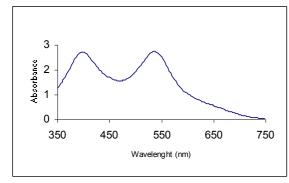
Figure 6. Absorption spectra of the Ruthenium complex dye
