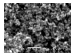
Figure 3. SEM picture of nanoporous TiO<sub>2</sub> film
