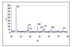
Figure 5. XRD pattern of TiO, film
