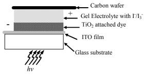
Figure 2. Structure of dye-sensitized solar cell
