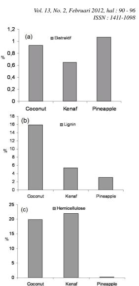
Coconut Kenaf Pineapple Figure 1. Chemical compositions (%) of three pulp fibers (a). Extractives, (b). Lignin, (c). Hemicellulose and (d). Cellulose
