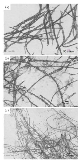
*Figure 3.* Optical microscopy images of three pulps fiber at 10X magnification (a). Coconut (b). Kenaf and (c). Pineapple pulps.
