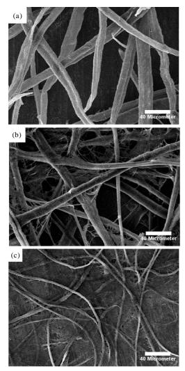
*Figure 4.* SEM image of three pulps fiber (a). Coconut (b). Kenaf and (c). Pineapple pulps
