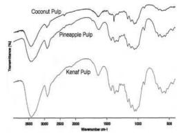
Figure 2. Infra red spectra of three pulps fiber.
