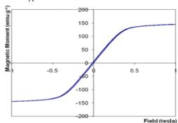
Figure 3. Hysteresis curve of the 24-chromium ferritic stainless steel found by VSM equipment
