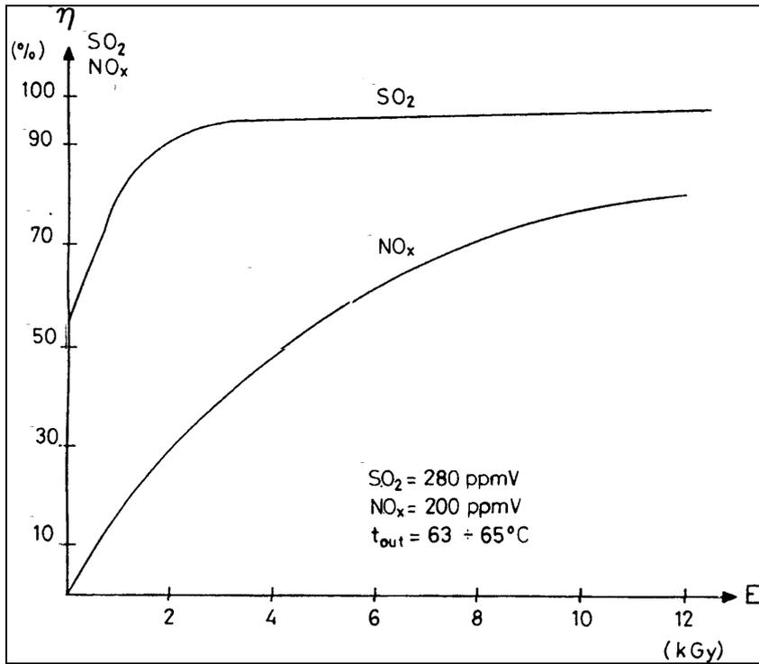
Gambar 5. Removal efficiency NO<sub>x</sub> dan SO<sub>2</sub> versus dosis<sup>[3]</sup>
